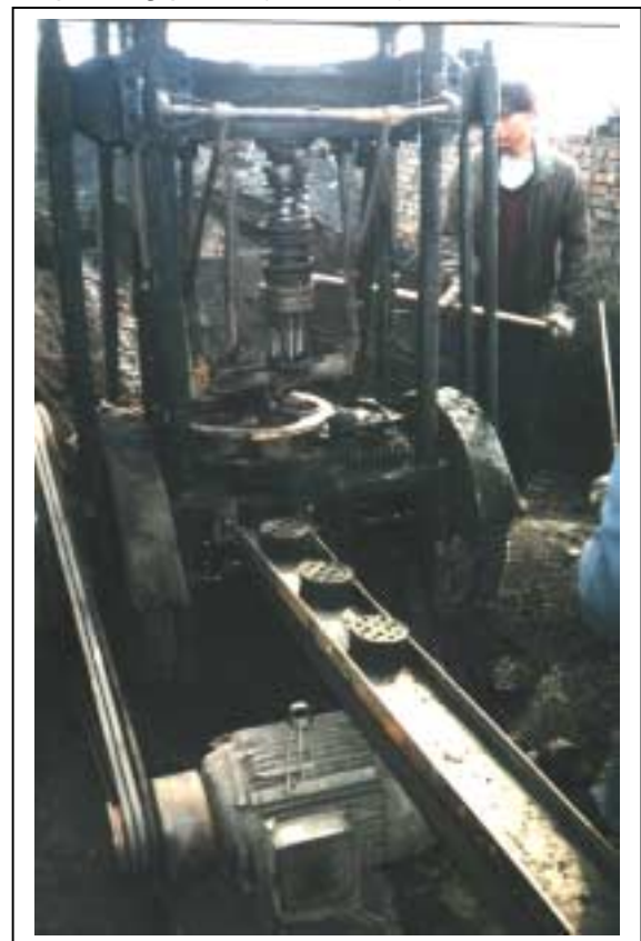
Pic. 8: Chinese semi-mechanised briquetting press /7/
