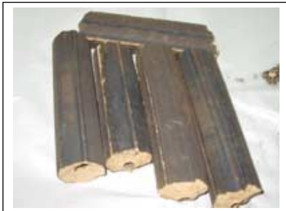
Pic. 4: Extruder briquettes from Thai Production /5/
