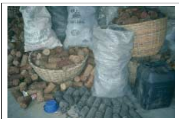
Pic. 10: Manually produced briquettes from biomass and waste paper in Benin /8/
