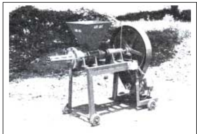
Pic. 2: Locally manufactured screw extruder from Thailand /5/
