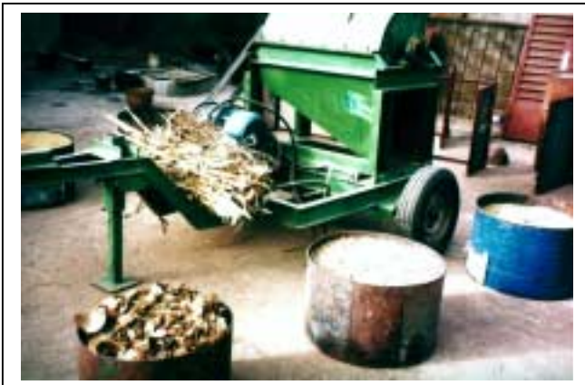
Pic. 1: Mobile shredder for agricultural residues from Mali /2/
