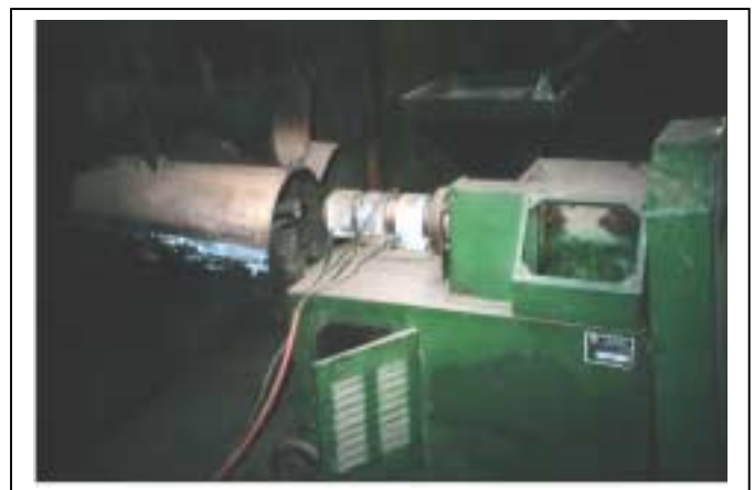
Pic. 3: Locally manufactured screw extruder from Mali /2/
