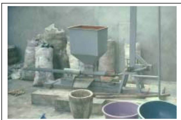
Pic. 9: Manual briquetting press for biomass and waste paper in Benin /8/
