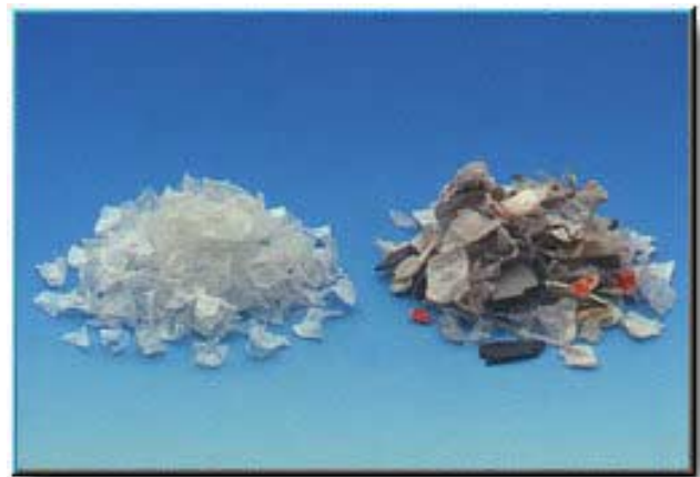
Fig. 11: Mixed and colour sorted PET-chips(flakes) after shredding, washing and fine separation
