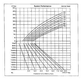
Figure 2: System performance curves (Source: GRUNDFOS)
