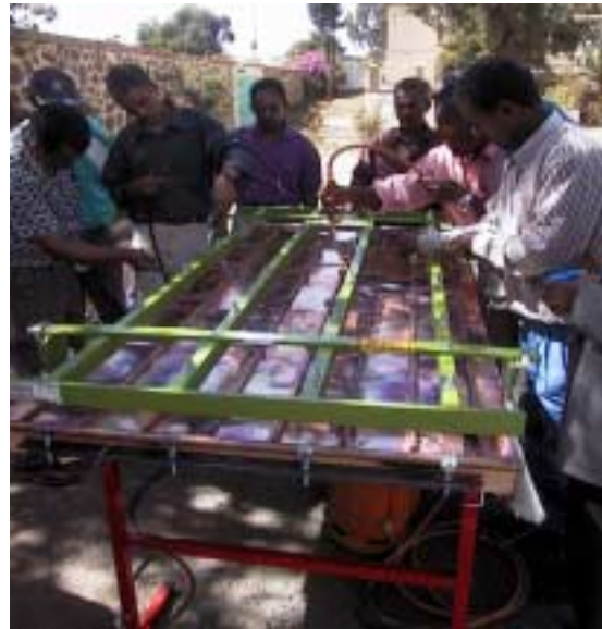
Fig. 4: soldering of the absorber on the soldering table.
