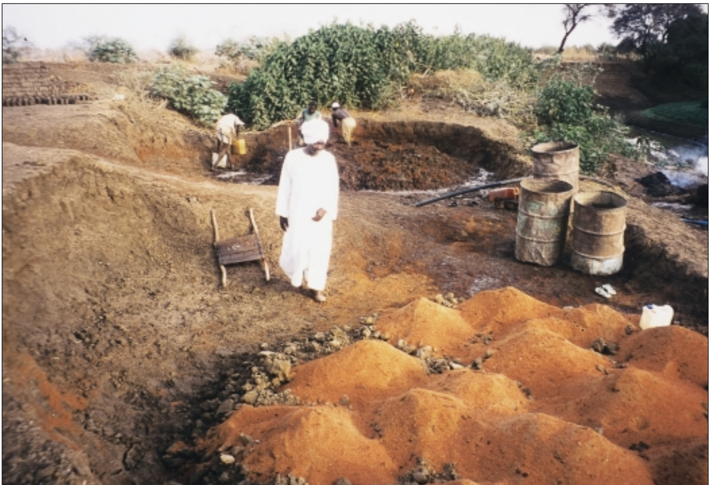
Fig. 1: Sawdust being used for fuel in brickmaking in Sudan. Note: Clay and sawdust are being mixed in the background.
