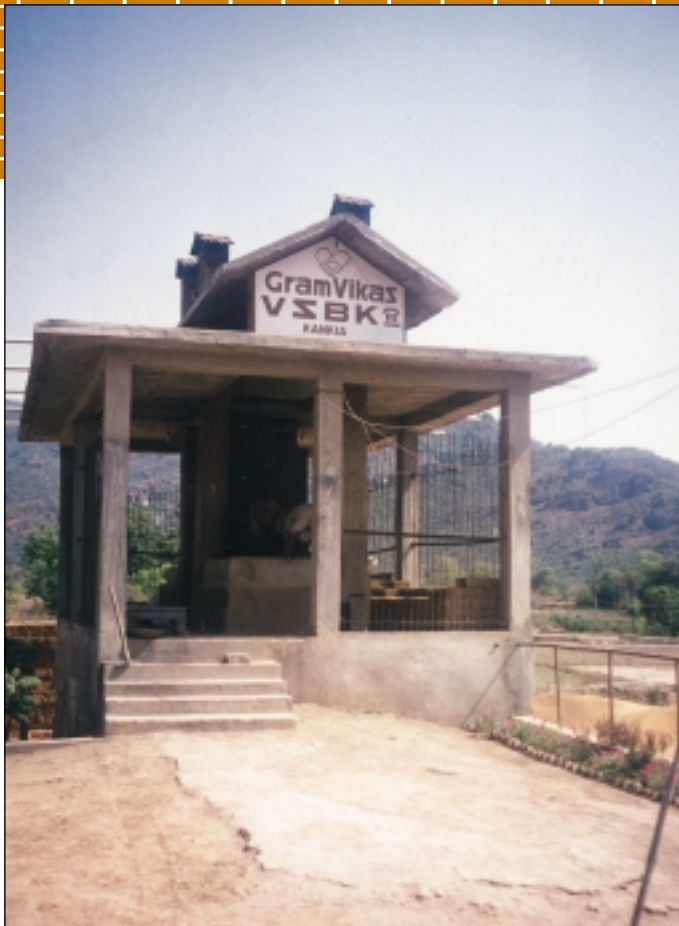
Fig. 2: An Indian vertical shaft brick kiln (VSBK). Trials with rice husks as fuel have been undertaken in this kiln.
