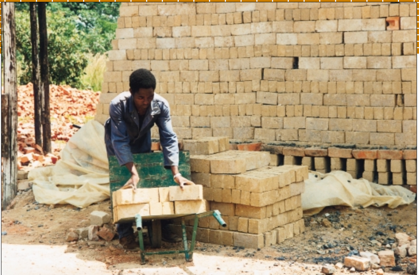
Fig. 4: Loading dried clay bricks into clamp for firing using boiler ash waste in Zimbabwe - by H. Schreckenbach
